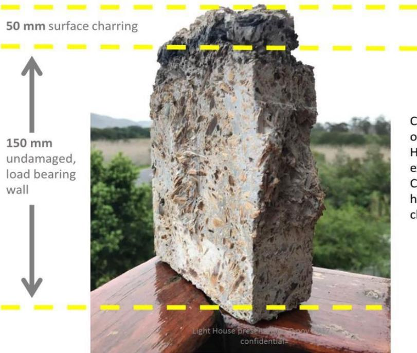
Cross-cut sample of 200mm Light House wall after exposure to 1 100 C furnace for 3 hours, 70% chipped gum trees
