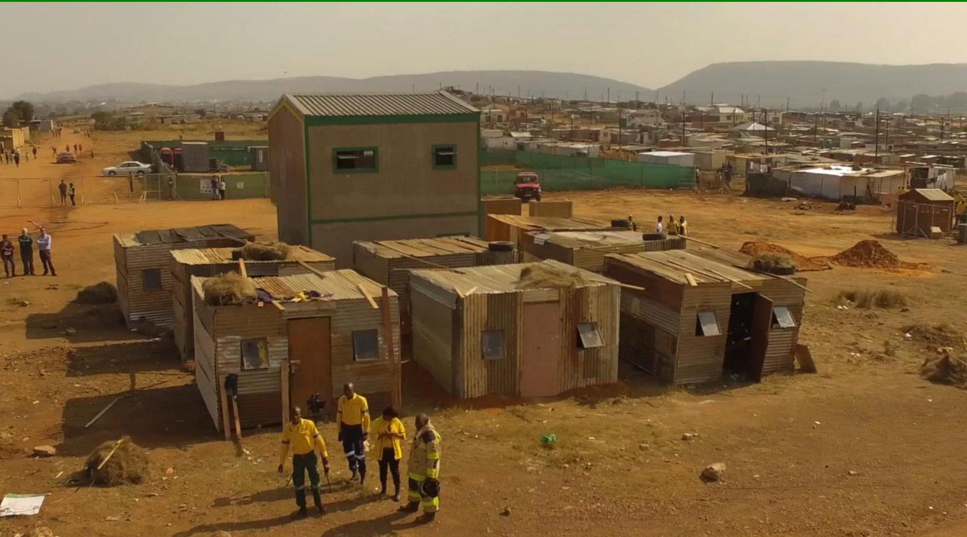
The successful fire-test in Mamelodi, testing woodwool-cement board. A Light House was surrounded by 8 shacks that were then incinerated. One of the shacks was lined with our material, and fire-shutters. Both the treated shack and the Light House were unscathed. The others were burned to the ground. Temperatures reached 1,500°C. We were so confident that we had people in the house during the fire.
