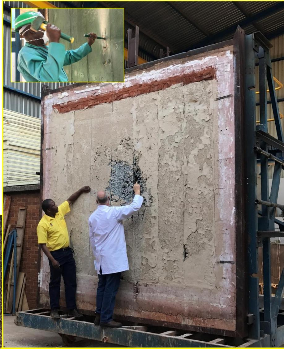
The Agrément certification has been achieved with flying colours – a three-hour fire-rating; three-story load-bearing, and superior properties shown overleaf. It was tested over 3 years to be termite-proof (left).
