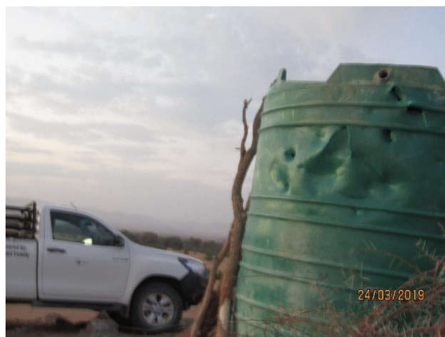
Water tank damaged by an elephant in Anabeb
