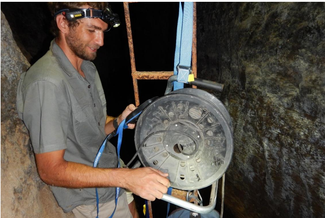
Figure 7: Measuring in situ water quality during both surveys using a Hach HQ40d portable multi-meter lower to 40 m whereby a reading was recorded every meter.
