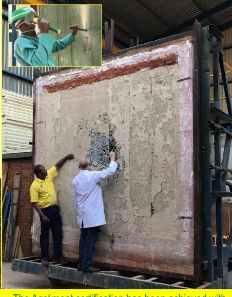
The Agrément certification has been achieved with flying colours – a three-hour fire-rating; three-story load-bearing, and superior properties shown overleaf. It was tested over 3 years to be termite-proof (left).
