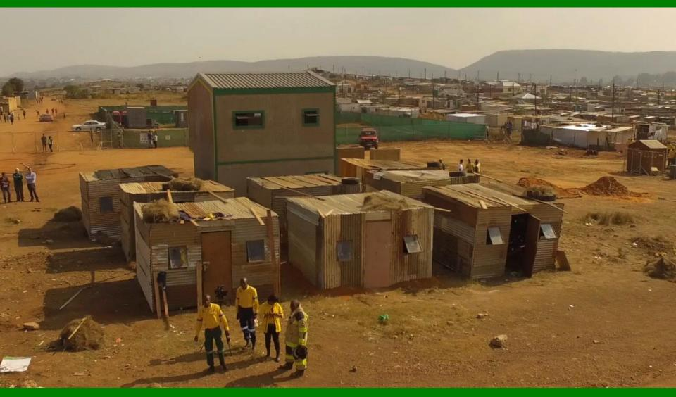
The successful fire-test in Mamelodi, testing woodwool-cement board. A Light House was surrounded by 8 shacks that were then incinerated. One of the shacks was lined with our material, and fire-shutters. Both the treated shack and the Light House were unscathed. The others were burned to the ground. Temperatures reached 1,500°C. We were so confident that we had people in the house during the fire.
