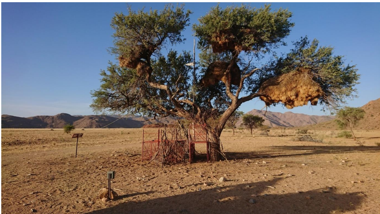
Figure 13: Electronic box traps targeting a coalition of territorial males. The traps were set on a farm in the Namib Desert. Notice the solar panel in the left and the directional antenna attached to a pole in the middle of the tree canopy.
