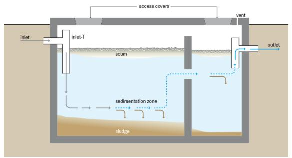
Schematic of a septic tank (https://en.wikipedia.org/wiki/Septic tank)
