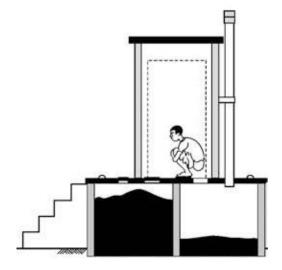
Elevated double vault pit latrine. This model can be used in flood prone areas or where groundwater is close to the surface.
