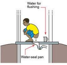
Design of squatting pan with water seal, pour flush system. (https://en.wikipedia.org/wiki/Pit\_latr ine)
